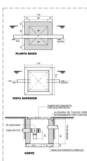
**CAIXA DE INSPEÇÃO SIFONADA (80 x 80 cm) SEM ESCALA**
