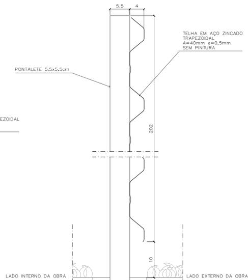
DETALHE 2: TELHA SOBRE PONTELETE
